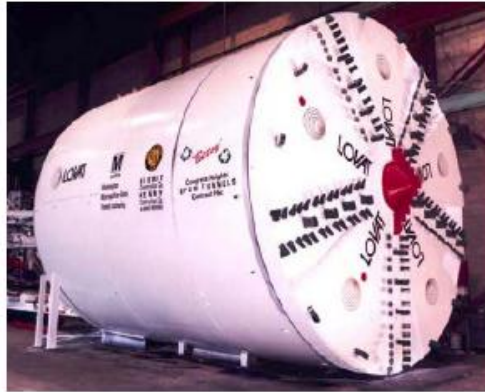
Earth Pressure Balance Tunnel Boring Machine (EPB) (Lovat).
