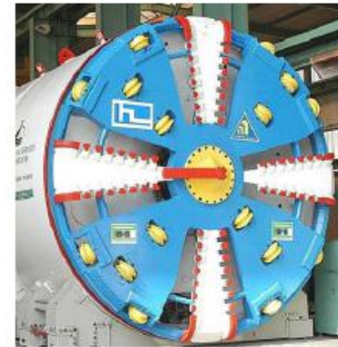
Slurry Face Tunnel Boring Machine (SFM) (courtesy of Herrenknecht).
