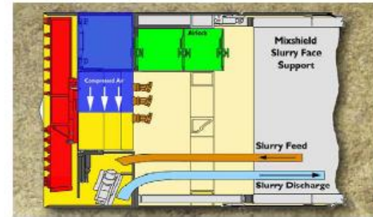
Simplified Cross-section of Slurry Face Tunnel Boring Machine (SFM) (from Herrenknecht).
